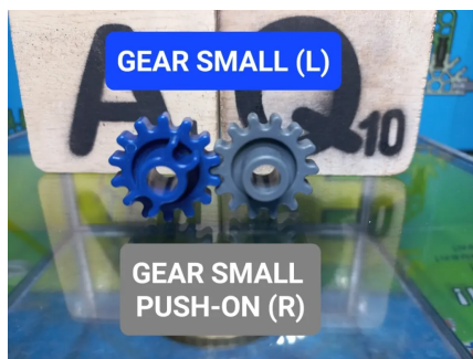
Small 14-tooth gears: standard and push-on
