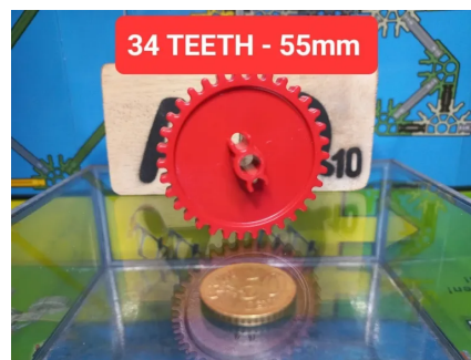
Medium gear: 34 teeth, about 2.2 in. (55 mm)
