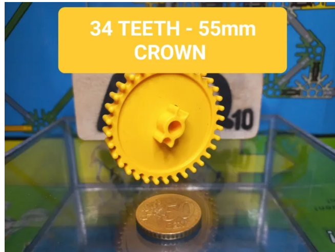
Medium crown gear: 34 teeth, about 2.2 in. (55 mm)
